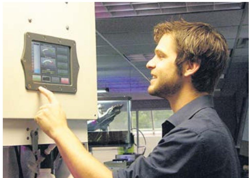
Robert Roulston demonstrates touch-screen controls on his new algae production unit. Operations can be fully pre-programmed or adjusted manually, and even monitored remotely via internet connection with a computer or cell phone.
