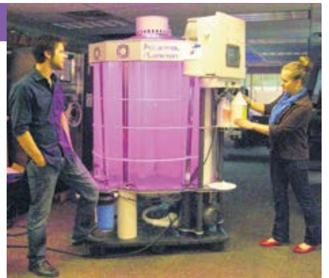
Robert and Ashley Roulston set up one of their Industrial Plankton Algae Bioreactor units for a test run. The self-contained unit will produce 1000L of algal suspension to a pre-set cell density in about a week, using either batch or continuous culture. And it's self-cleaning!
